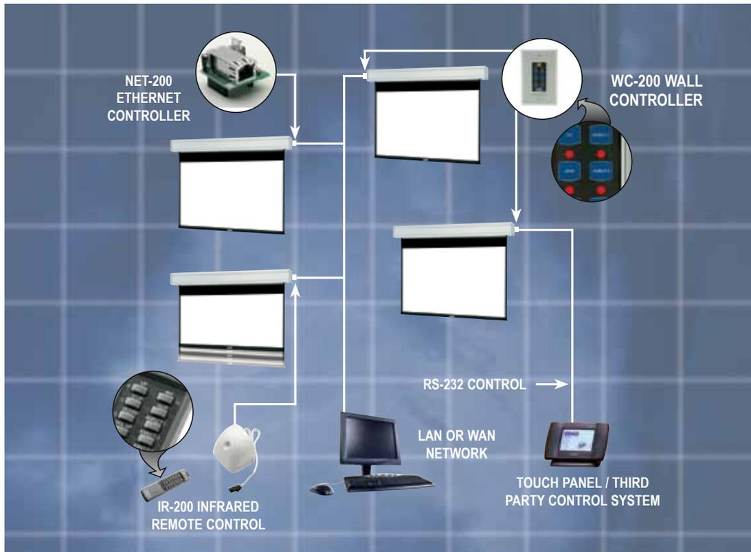
The SCB-200 screen controller provides control over a screen using RS-232C communications or an optional Ethernet controller, wall controller or infrared controller. Designed for applications where precise screen control and monitoring capabilities are crucial, the SCB-200 is available as a factory-installed option in the Contour, Tensioned Contour, Advantage, Tensioned Advantage, Advantage Deluxe, and Tensioned Advantage Deluxe.
