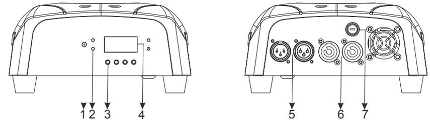
1. IR receiver: To receive the IR signal;
