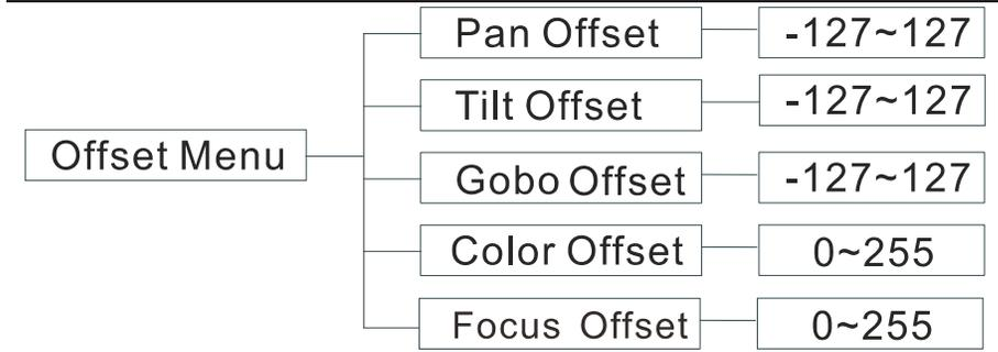
To enter the Offset Menu, press the MENU button to unlock the display, then press the ENTER button for at least 5 seconds. In this submenu you are able to adjust the home position of the pan, tilt, gobo wheel, color wheel, and focus. To exit this menu press and hold the MENU button.
