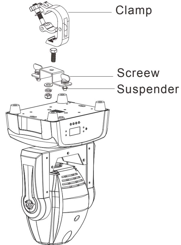
Screw one clamp via a M12 screw and nut to the included bracket. Attach the bracket using the omega locks to the bottom of the Focus Spot One. Attach and pull the safety-cable through one of the safety holes located on the bottom base and over the trussing system or a safe fixation spot. Insert the end in the carabine and tighten the safety screw.
