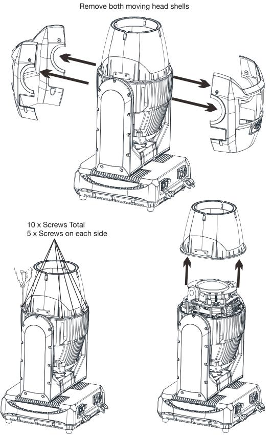
After the moving head shells have been removed unscrew and remove the 10 screws that secure the head in place. Carefully remove the head to access the inside module.
