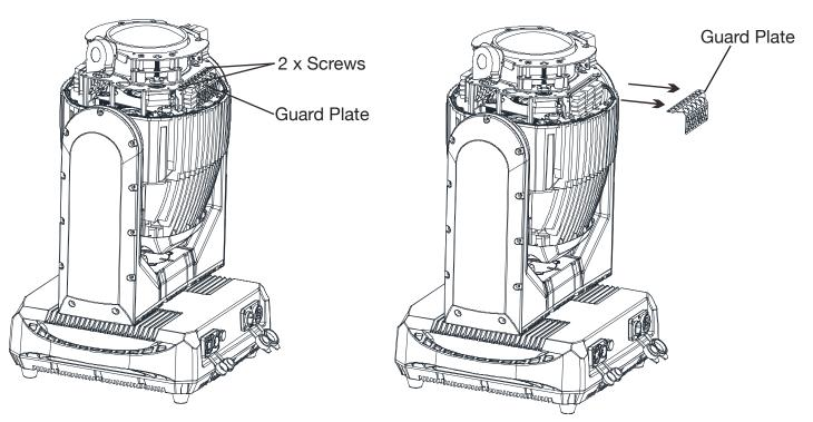
Note: Disconnect the cables with RED sleeves before dismantling head module.
