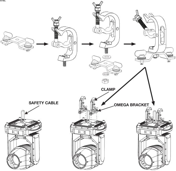
Screw one clamp via a M12 screw and nut into the Omega holder. Insert the quick-lock fasteners of the Omega holder into the respective holes of the adjustable mounting bracket. Tighten the quick-lock fasteners fully clockwise. Pull the safety-cable through the opening located on the bottom of the unit and over the trussing system or a safe fixation spot. Insert the end in the carabine and tighten the safety screw.
