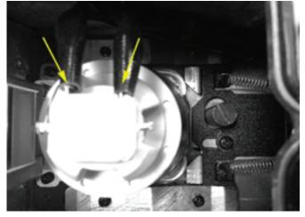
3. Gently remove the (2x) spade terminals connected to the lamp.
