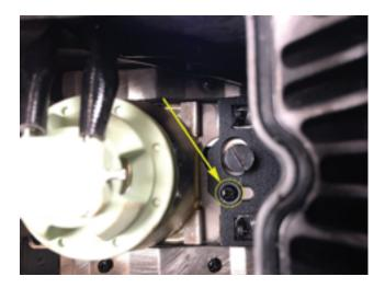
6. Once the new lamp has been inserted, loosen the Phillips head screw again to allow the lamp holding mechanism to slide back to its closed position. Tighten the Phillips head screw.
