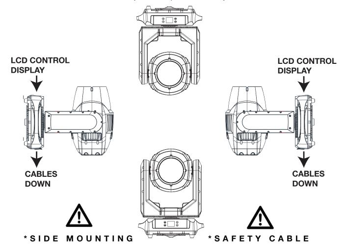
TO MAINTAIN IP65 RATING INTEGRITY, FIXTURE MUST BE INSTALLED WITH CABLES FACING THE GROUND AT ALL TIMES. WATER MUST EASILY RUN OFF AND NOT COLLECT AROUND CABLE CONNECTIONS.
