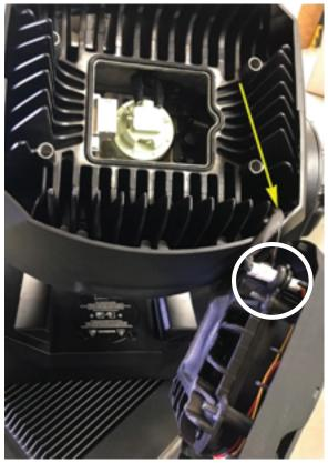
2. Unscrew the (4x) allen head screws to remove the rear cover. When removing the rear cover, please be advised that the cover is connected to the unit via a safety cable and connected wire cable.
