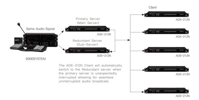
• The probability is a network data error when a using a single server is 1/1000 when a redundant server the data error probability is reduced to 1/1,000,000.
