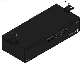
3 Mount the unit using the circular holes, on each mounting plate. If using a drywall surface, a #6 drywall screw is recommended. Mounting screws are not included.
