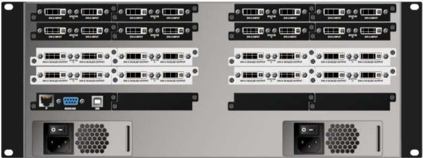
Standard Unit with 16 DVI-U Inputs and 16 DVI-U Outputs
