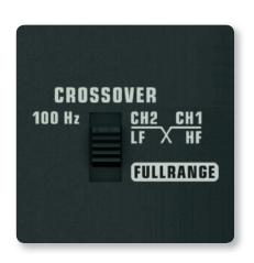
securely connect speakers. The same panel contains the switches that put the EPQ2000 in Mono, Stereo (two channel mode) or mono Bridge mode. A built-in Crossover switch allows you to send low-frequency content to subwoofers and other sound reinforcement speakers (CH1 < 100 Hz / CH2 > 100 Hz or Fullrange). Flick the Limiter On/Off switch to activate the built-in overload protection.
