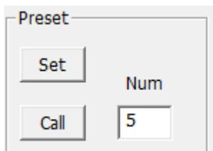
5. Press “Call” with the previously entered number in the “Num” field, and the camera will return to the original viewing area.
