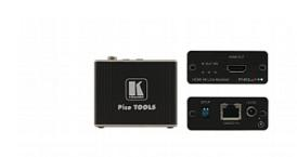
PT-872xr is a high-performance, long-reach DGKat™ 2.0 receiver for 4K@60Hz (4:4:4) HDR HDMI 2.0 and HDCP 2.2 signals and 2-way powering over twisted pair. It converts the transmitted DGKat™ 2.0 signal into an HDMI signal. PT-872xr extends the signal to up to 60m (200ft) at 4K@60Hz (4:4:4) resolution and up to 70m (230ft) at 4K@30Hz (4:4:4) 24bpp resolution over Kramer shielded cables. NOTE: To reach the distances listed, Kramer UNIKAT non-plenum bulk cable or pre-made assemblies MUST be used
