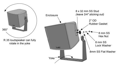
Mount yoke to the surface using holes aligned with large center hole as primary mounting points - these are aligned with the center of gravity. Use other holes as secondary reinforcement. Orient angled side to the front of the loudspeaker if the yoke is mounted below the enclosure.
