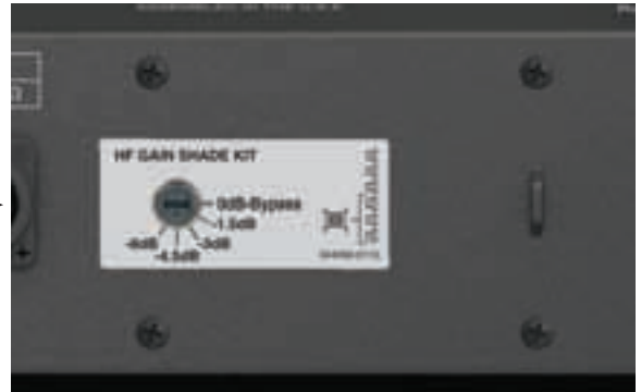
Figure 2. Installed RMSHADE Kit
