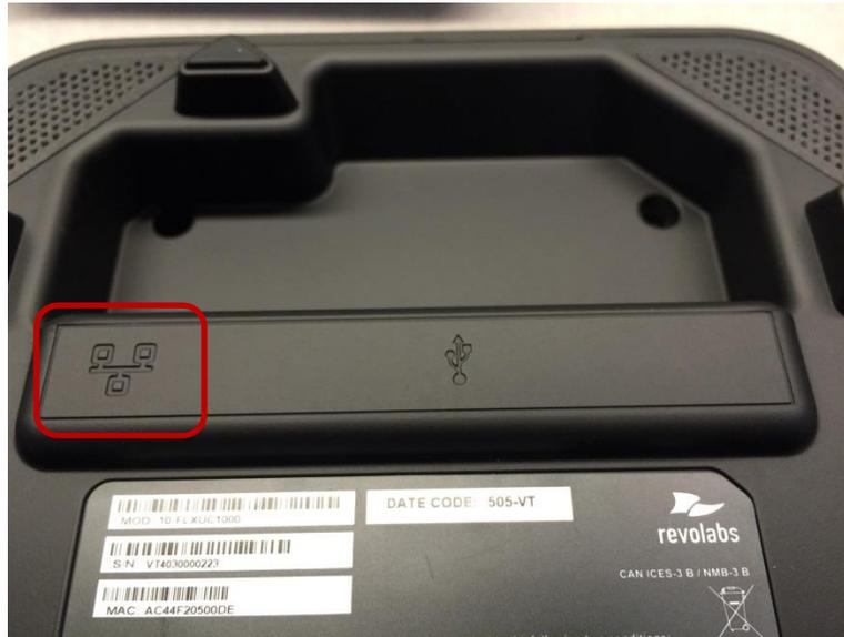
Connect one end of the Ethernet cable into the network connection port on the bottom of the base unit using the port highlighted in the picture above. Press the Ethernet connector until it clicks into place. Connect the other end of the Ethernet cable into a jack providing PoE or a PoE adapter.
