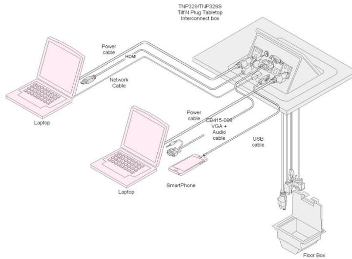
Diagram 1: Typical Setup and use of a TNP329
