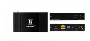
TP-874xr is a high-performance, long-reach DGKat<sup>™</sup> 2.0 receiver for 4K@60Hz (4:4:4) HDR HDMI HDCP 2.2 signals, RS-232 and IR signals and 2-way powering over twisted pair. It converts the transmitted DGKat<sup>™</sup> 2.0 signal into an HDMI, RS-232 and IR signals. TP-874xr extends the signal to up to 50m (160ft) at 4K@60Hz (4:4:4) resolution and up to 70m (230ft) at 4K@30Hz (4:4:4) 24bpp resolution over Kramer shielded cables
