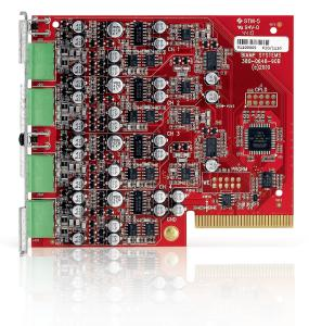
The Tesira<sup>®</sup> SIC-4 is a modular analog input card for use with Tesira SERVER and SERVER-IO devices. Each SIC-4 provides 4 channels of Mic or Line level audio input. The inputs are electrically balanced and provided on plug-in barrier strip connectors. Software control of each input includes gain with clip indicator, +48V phantom power, mute, level and signal invert.
