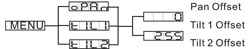
To enter the Offset Menu, press the ENTER button for at least 3 seconds. In this submenu you are able to adjust the home positions of the pan & tilt motor.
