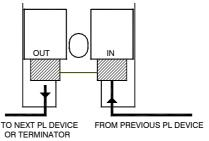
End of chain termination As with any RS485 system, the last PL device needs to have a terminating resistor fitted to its output port. Early version PL-4 modules are shipped with a 100 ohm resistor already fitted. Leave this fitted only if the unit is the last in the chain. Later version PL-4 modules are supplied with a terminating RJ45 plug (Allen & Heath part number 003-082).
