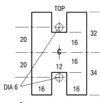
The assembled module fits into an 'H' shaped cutout in the centre of the mounting plate. The module is held using the two screws with plastic clamps provided (A). Unscrew these from the module first. Dimensions are in millimetres below.
