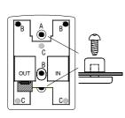
To change them, first remove the three screws (B) and unplug the top PCB. Remove the three screws (C) and lift the lower PCB away. Rotate the switch caps into the required position. Reassemble the module taking care to correctly align the inter-PCB connector.
