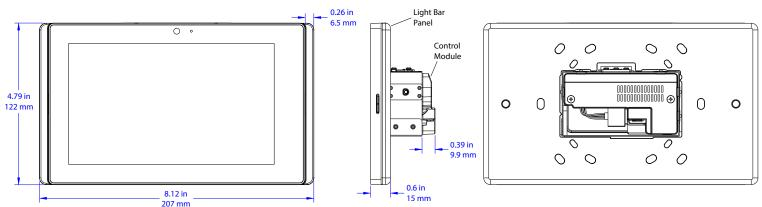
TSW-760-LB light bar assembly shown installed on a TSS-7 or TSW-760 touch screen
