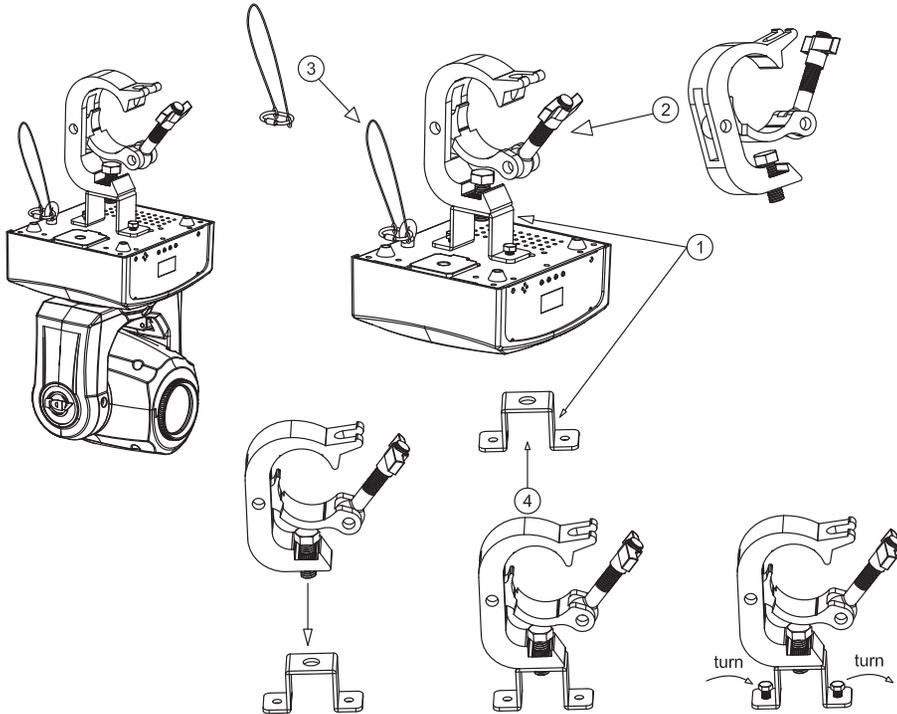
Screw one clamp via a M12 screw and nut to the included bracket. Attach the bracket using the included screws to the bottom of the Stinger Spot. Attach the eyehole screw to the bottom of the base and pull the safety-cable through the screw and over the trussing system or a safe fixation spot. Insert the end in the carabine and tighten the safety screw.
