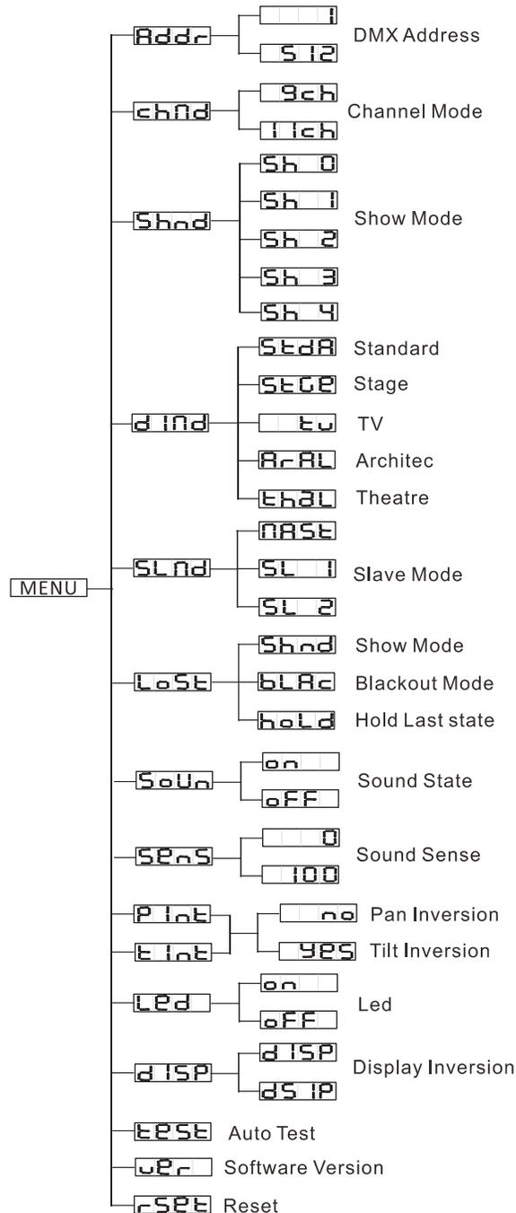
**System Menu:** When making adjustments press **ENTER** to confirm your setup then press and hold the **MENU** button for at least 3 seconds. To exit without making any adjustments press the **MENU** button. The display will lock after 30 seconds, press the **MENU** button for 3 seconds to unlock.
