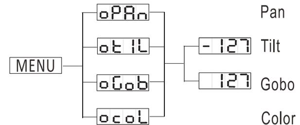
To enter the home position adjustment menu, press the ENTER button for at least 5 seconds. In this submenu you are able to adjust the original position of the pan position, tilt position, color wheel position, and gobo wheel position.
