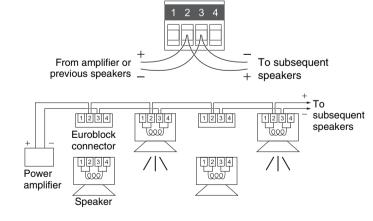
4 Plug the connected Euroblock connector into the socket in the
