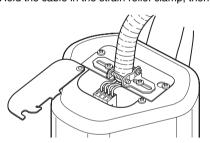
8 Close the terminal cover and tighten the screw.
