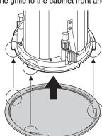
The grille may fall down if it is attached inadequately. Attach it firmly
